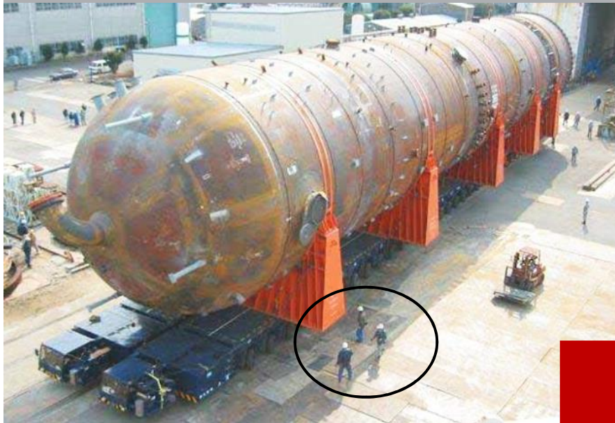
Conventional Fischer-Tropsch reactor
