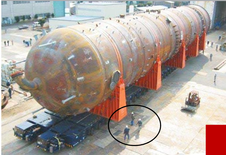
Conventional Fischer-Tropsch reactor
