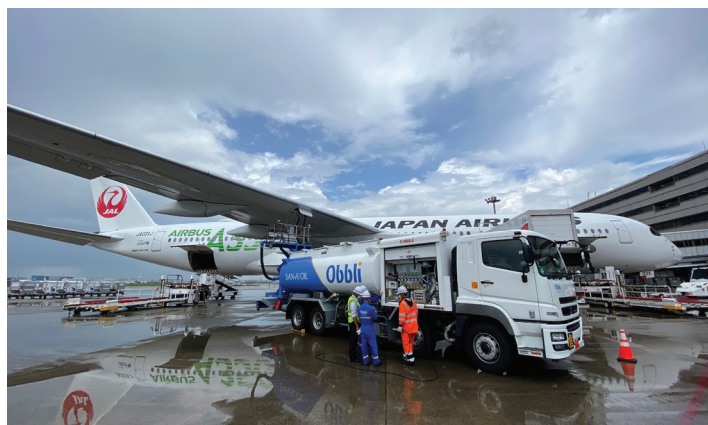
Fuelling JAL flight with SAF at Tokyo Haneda Airport. Photo courtesy of NEDO.
